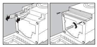
Set the machine upright and remove the two remaining bolts from the back.
